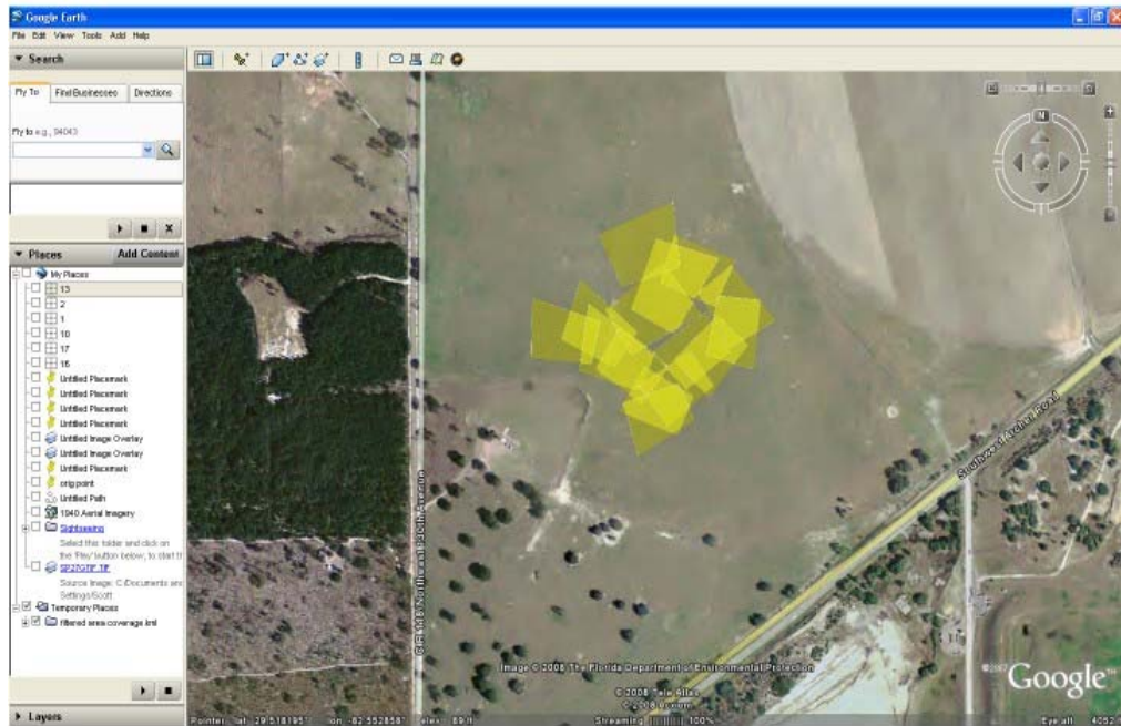
Figure 7-8. Example of area coverage assessment generated from PolarisView. These yellow overlays represent estimated photographed area at time of exposure.
