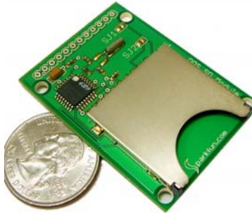
Figure 4-9. DosonChip SD Memory Card hardware used to store synchronized UAV orientation and location data
