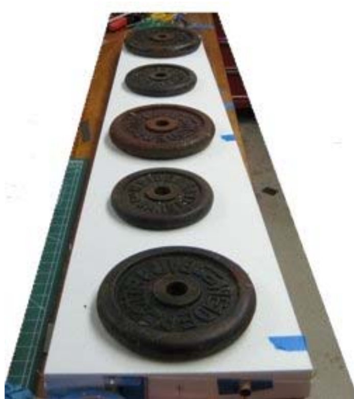
Figure 3-4. Process for compressing fiberglass curing epoxy to EPS foam wing cores
