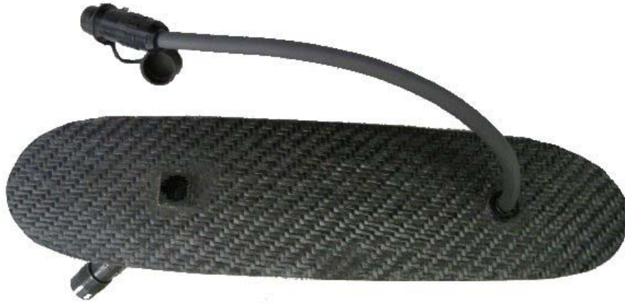
Figure 3-5. Saddle hatch for programming access of PDIB processor and wing connectivity
