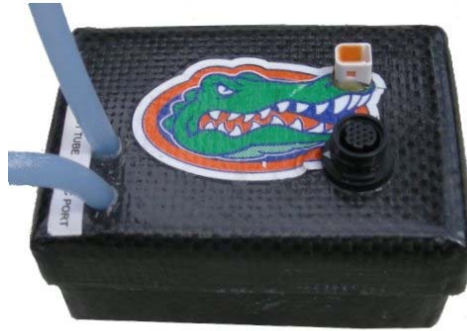
Figure 4-3. Carbon fiber box for autopilot with waterproof interfacing electrical connectors
