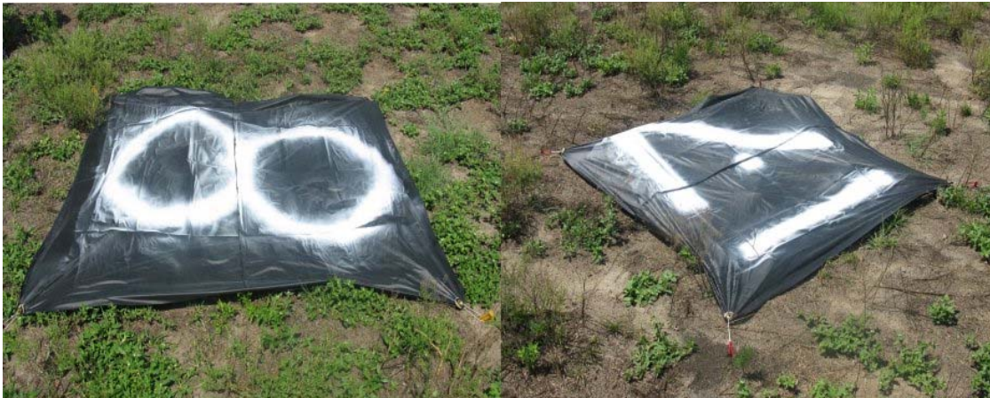
Figure 8-1. Examples of ground control targets used for spatial comparison in the mapping process. Targets are 1.5 meters square. A) Target 8 B) Target 17
