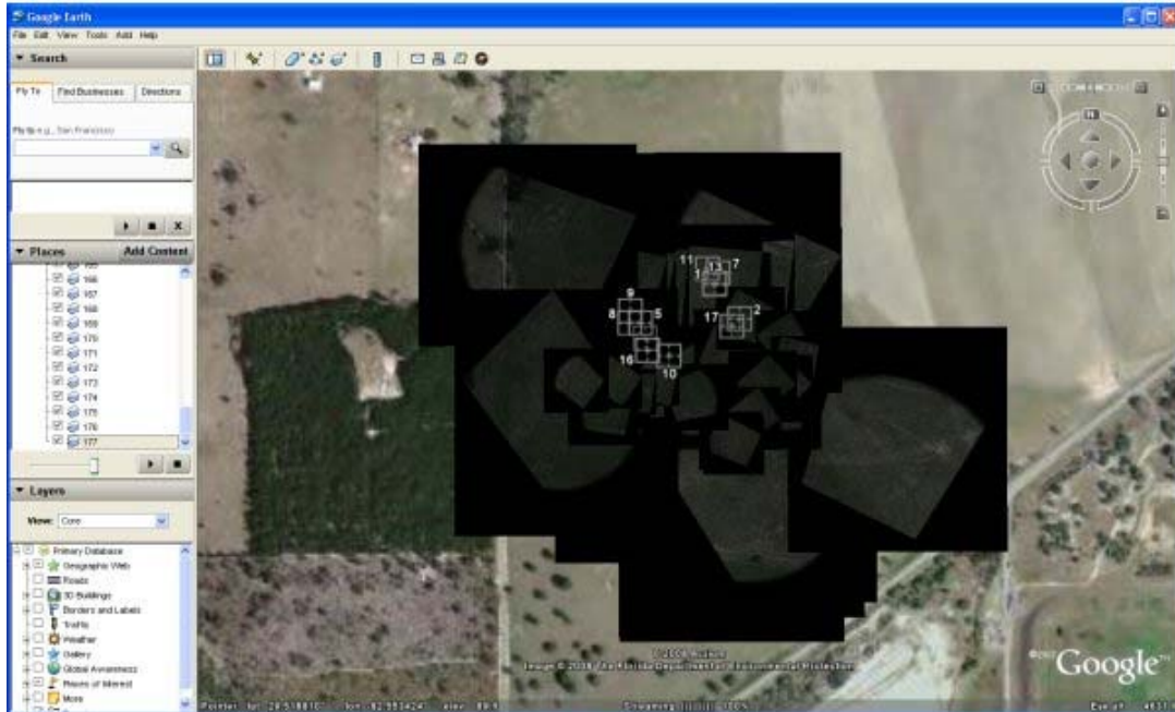
Figure 8-3. Rectified images for data set are rectified and registered from PolarisView into Google Earth®'s interface
