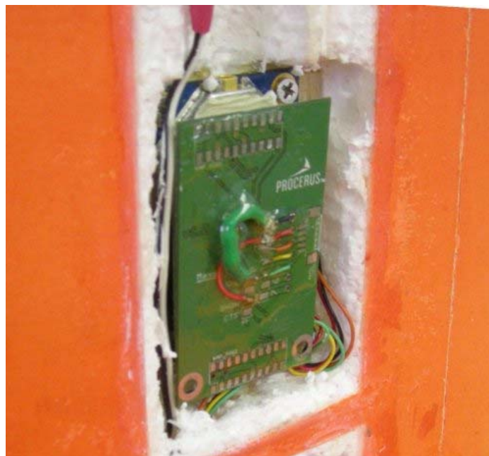
Figure 4-2. One Watt Aerocom modem is mounted in tail to reduce EMI
