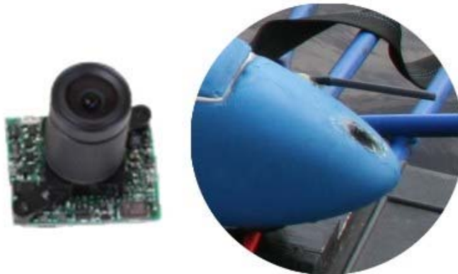
Figure 4-10. KX-141 CCD camera and installation location
