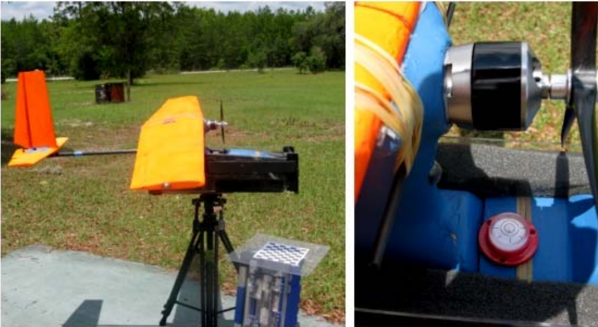
Figure 6-7. Field initialization process for determining camera boresight misalignment A) Initialization Jig used for extracting exterior calibration parameters. B) Bubble leveling technique used to ensure orthogonality between calibration grid and UAV.
