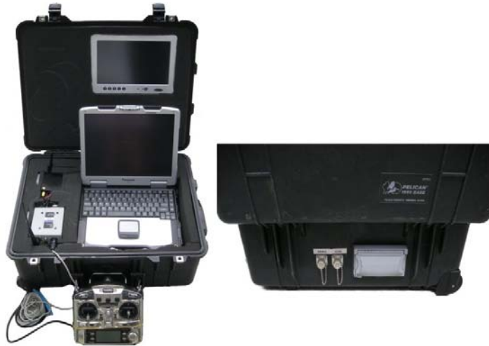
Figure 4-15. Front and back of Ground Control Station (GCS)
