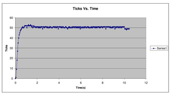
The settling time was ~.3 seconds and there was nearly no overshoot. The graph shows ticks of my homemade encoders over a period of 50 ms. The controller was designed to stay at 50 ticks. I have since overhauled my controllers by switching to fixed point math. I also am now using an output compare interrupt to trigger the PD corrections.
