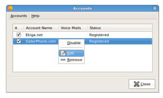
10. This opens up the "Edit Account" window in which we can modify the parameters such as user-id, SIP server name, password, timeout etc.,
