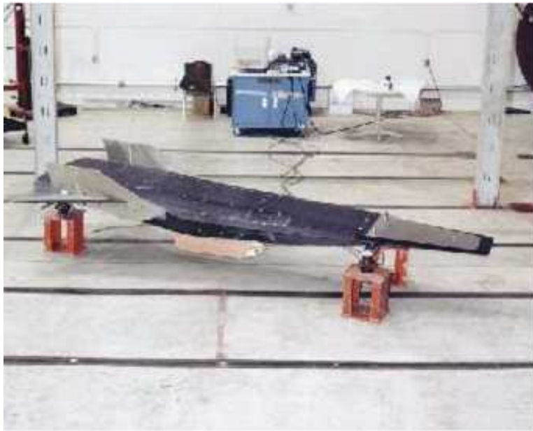
Figure 1-2. The X-43 model during GVT
