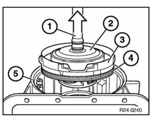
14. Remove the overrun sub assembly along with the 4th clutch plates.
