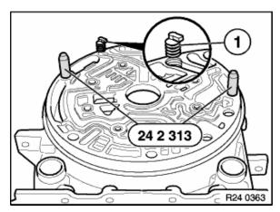
24. Insert (Transfer Plate Guides) special tools 24 2 313 on the adapter case as shown.
