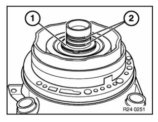
33. Install 2 new seal rings and thrust washer using petroleum jelly.
