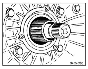
6. Apply petroleum jelly or transmission fluid to the new radial seal ring and install. Tighten the three screws to 3 Nm (2.2 lb.ft.).
