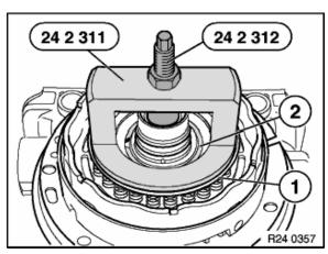
32. Install tool 24 2 311 onto the center support. Using tool 24 2 312, compress the relief springs, the seat, and the snap ring. **DO NOT OVER COMPRESS-RISK OF BENDING THE SPRING SEAT.**Install the snap ring in the groove using a snap ring pliers. **ENSURE THE SNAP RING IS CORRECTLY IN PLACE.**Release the pressure and remove the special tools.
