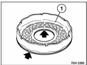
27. Install new inner and outer seals on clutch piston (1).
