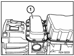
7. Rotate transmission 180( so that the oil pan is facing up. Remove the front oil pan and gasket after removing 12 screws.
