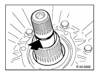
10. Remove 'O' ring seal from turbine shaft end.
