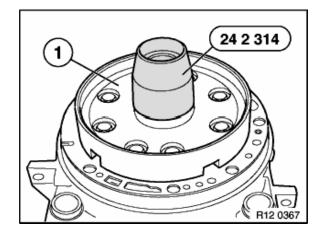
28. Place (Clutch Piston Installer Sleeve) special tool 24 2 314 over center support (1) hub as shown.
