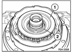
31. Install seat (1) on relief springs. Place the new snap ring (2) on the seat.
