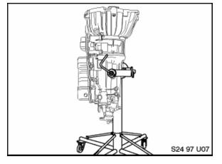
9. Rotate transmission 90( so that converter housing is facing up.
