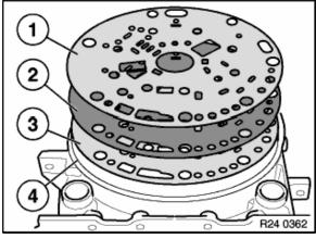
23. Remove gasket (1), Transfer plate (2) and gasket (3). Discard the two gaskets.
