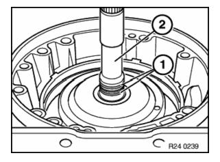
13. Remove the two teflon seal rings (1) on the turbine shaft (2).
