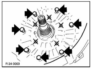
11. Remove the 7 bolts holding the converter housing to the adapter case.
