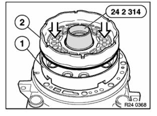
29. Install the reverse clutch piston (2) over center support (1). Remove tool 24 2 314.
