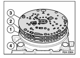
25. Install gasket (1), transfer plate (2), and gasket (3) to adapter case (4).
