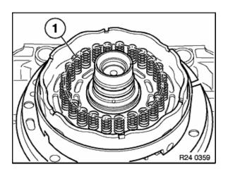
30. Install the 24 relief springs (1) on reverse clutch using petroleum jelly.
