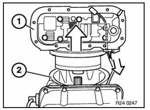
17. Slowly remove the adapter case (1) to ensure that the 3rd clutch shaft is not displaced. **NOTE:** The wiring harness attached to the valve body main case must be fed through the hole in the adapter case as it is being removed.
