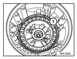
16. Remove the thrust washer(1).
