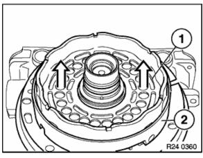
18. Turn adapter case upside down. Compress seat (1) using tool 24 2 311 and 24 2 312 or a press. Remove snap ring (2) from groove using snap ring pliers. Release the tool and remove.
