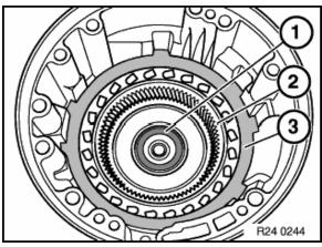
15. Remove the following: Last 4th clutch plate (3). Thrust bearing (1), note the position of the bearing (black side up). Overdrive ring gear (2).
