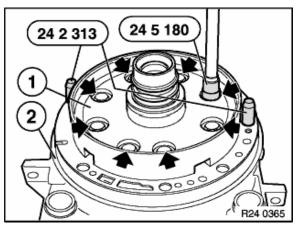
26. Install center support hub (1) with 8 screws. Tighten progressively to 25 Nm.
