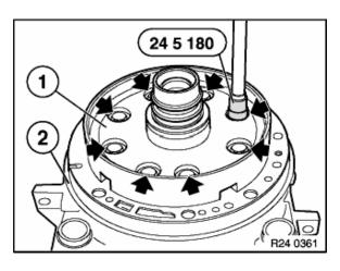
22. Unscrew 8 screws (1) from center support (2). Remove center support from adapter case.
