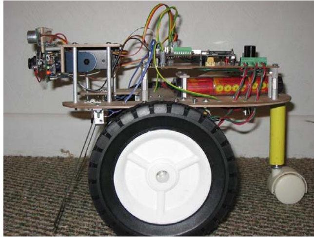
Figure 3 - Showing battery, servo, bump switches
