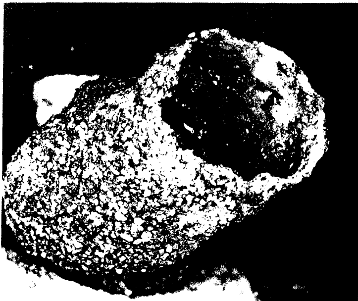
Figure 2: A sand fulgurite made by triggered lightning in 1993 at Camp Blanding
