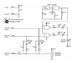
Though the device can detect objects in 3 different cones as the picture below shows, there is only 1 sensor output signal that goes low when an object is detected and is high otherwise. Alternating the LED enable signals will allow the microcontroller to distinguish which cone the object is in.
