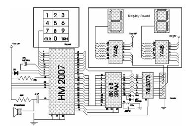
In order to test this circuit I trained the device with the different words I will need my robot to recognize:
