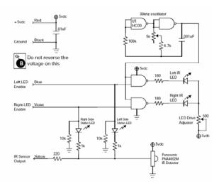
Though the device can detect objects in 3 different cones as the picture below shows, there is only 1 sensor output signal that goes low when an object is detected and is high otherwise. Alternating the LED enable signals will allow the microcontroller to distinguish which cone the object is in.
