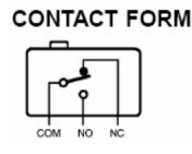
The signal line that is sent to the microcontroller will be connected to the COM terminal with a resister in series, the NC terminal will be connected to GRND, and the NO terminal will be connected to VCC. This connection will ensure that when the cards are placed in the loader +5V will be sent to the microcontroller. I wired up the 2 sensors and
