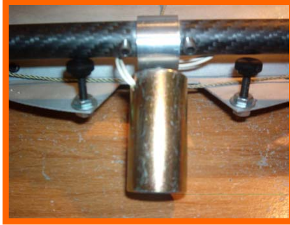
Figure 8. Magnet Mount, Collar and Wire Route
