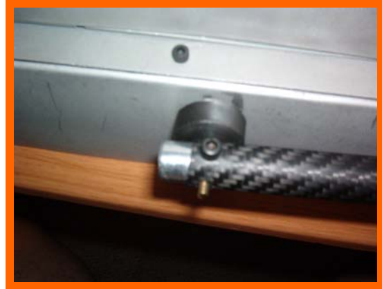
Figure 6. Rear Arm Detail with Nylon Spacer
