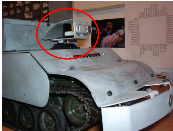
Figure 3. SRF08 Mounting Location
