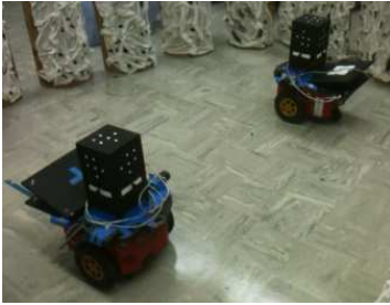
Fig. 7. Two Pioneer P3-DX robots equipped cameras and targets. Robot 1 is shown on the left, while robot 2 is on the right.
