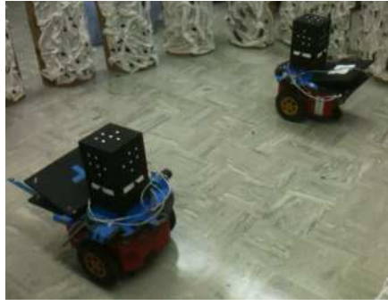
Figure 9: Two Pioneer P3-DX robots equipped with cameras and targets. Robot 1 is shown on the left, while robot 2 is on the right.
