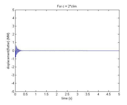
C) Here we see that as c increases the system stability increases. Specifically when c < clim, the system is extremely unstable and the flutter increases gradually with time. At c= clim, this is the critical damping limit and at this point the the flutter is constant. As c increases and it gets more than clim, the system gets stable. Initially there is some flutter and it gets stable gradually with time.
