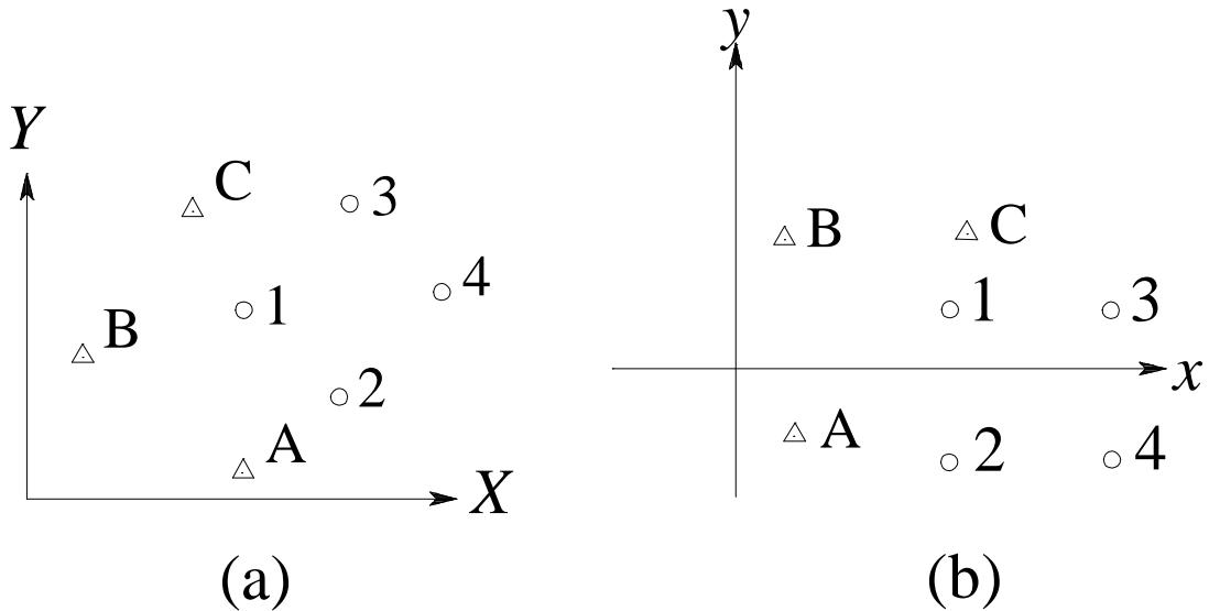
Steps in transforming coordinates measured in the coordinate system shown in (b) into that shown in (a).
