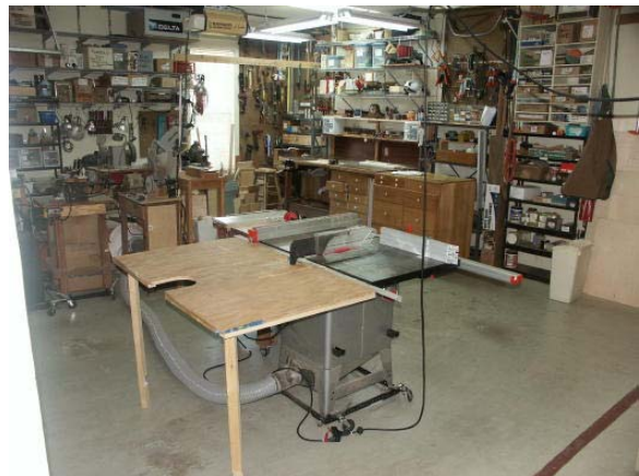
Figure 1 Folding outfeed table and side table for saw and rolling tool cabinets (background). The cabinet under the bench rolled out to give access to shelves behind it.
