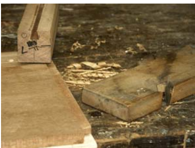
Figure 1. Apron on shooting board with dovetail plane, leg in background
