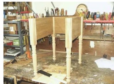
Figure 3. Dry- assembled Table Stands Without Clamps
