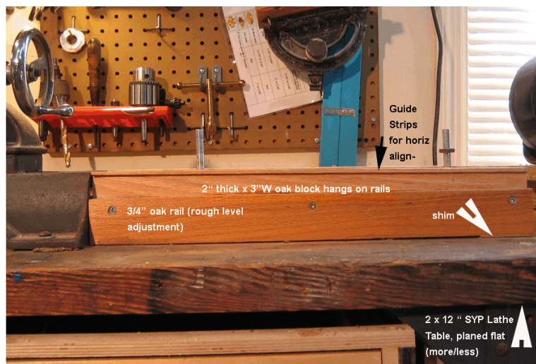
Figure 2. Side View of Bed Extension. End of iron lathe bed appears at the left.
